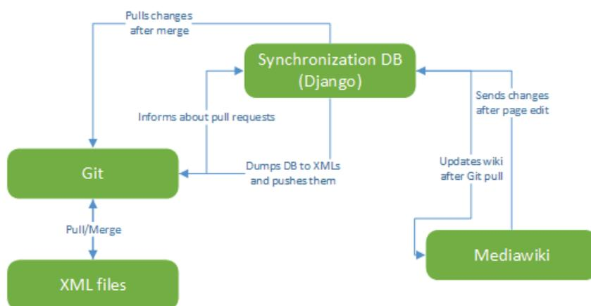
Figure 2: System architecture
